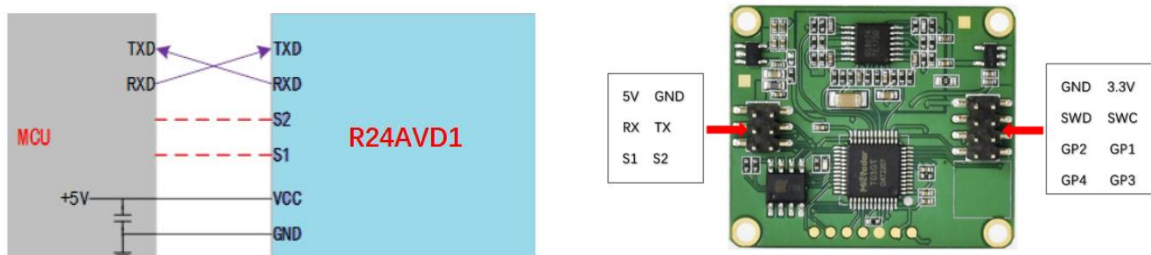
Fig. 4: Schematic diagram for connection between radar module and peripherals
