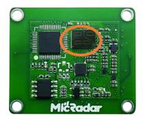
The part enclosed in yellow is the radar antenna
