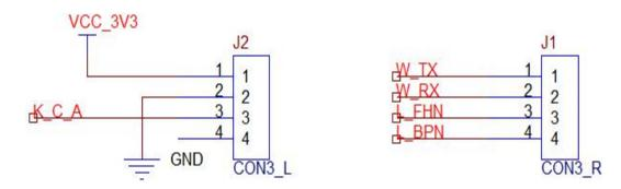
If the silk screen of the board is the same, W\_TX and W\_RX are the serial ports of the connection module, and L\_FHN and L\_BPN are the IO of the connection module respectively.
