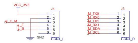
If the silk screen of the board is the same, M\_TX0, M\_RX0 are MCU serial port 1, M\_TX1, M\_RX1 are MCU serial port 2, M\_SDA, M\_SCL are the light sensor driver interface (IIC)
